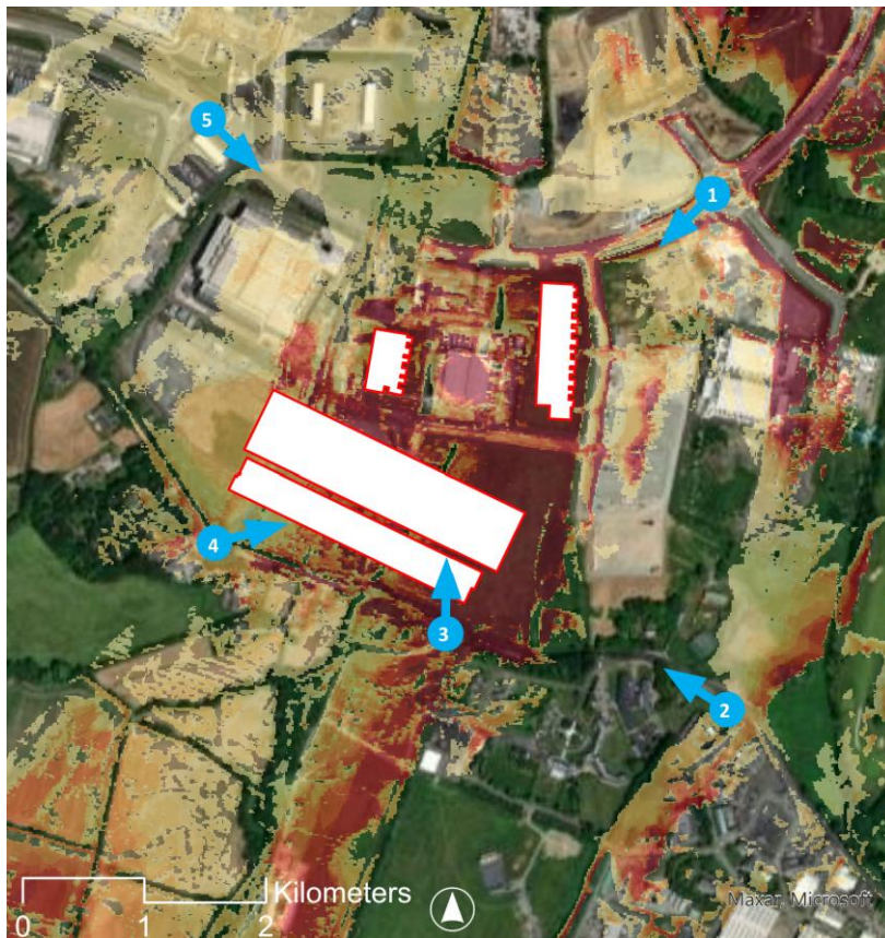
Figure 15.4: Viewshed generated from GIS using a Digital Terrain Model illustrating the ZTV.
